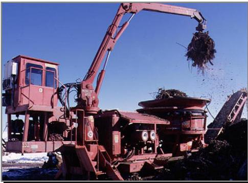
Volumes of raw organic materials can be ground quickly, making the operations very cost competitive. The reduction of volume translates into reduced transportation costs. Finally, the ground material can either be used as mulch or it can be composted.
